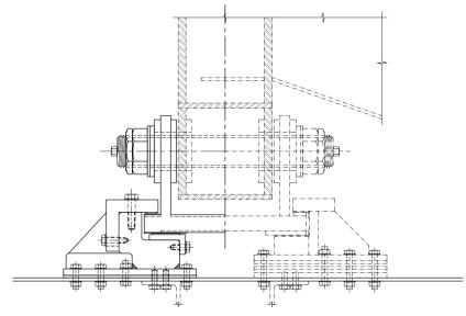
Figure 3. New bearing (left, solid lines) and previous bearing (right, dashed lines) geometry.
