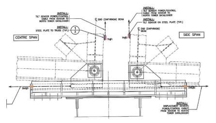
Figure 10. Location of the displacement sensor on bearings.
