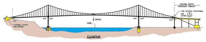
Figure 1. Lions Gate Bridge Suspended Spans Elevation.
