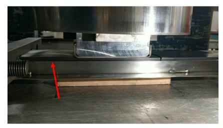
Figure 7. Testing a UHMWPE specimen to buckling failure.
