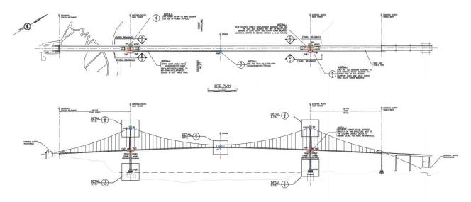
Figure 8. Instrumentation layout.
